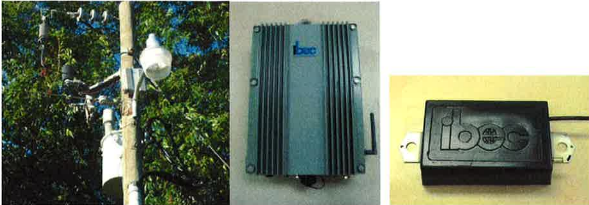
IBEC BPL REGENERATOR & CUSTOMER ACCESS UNIT
